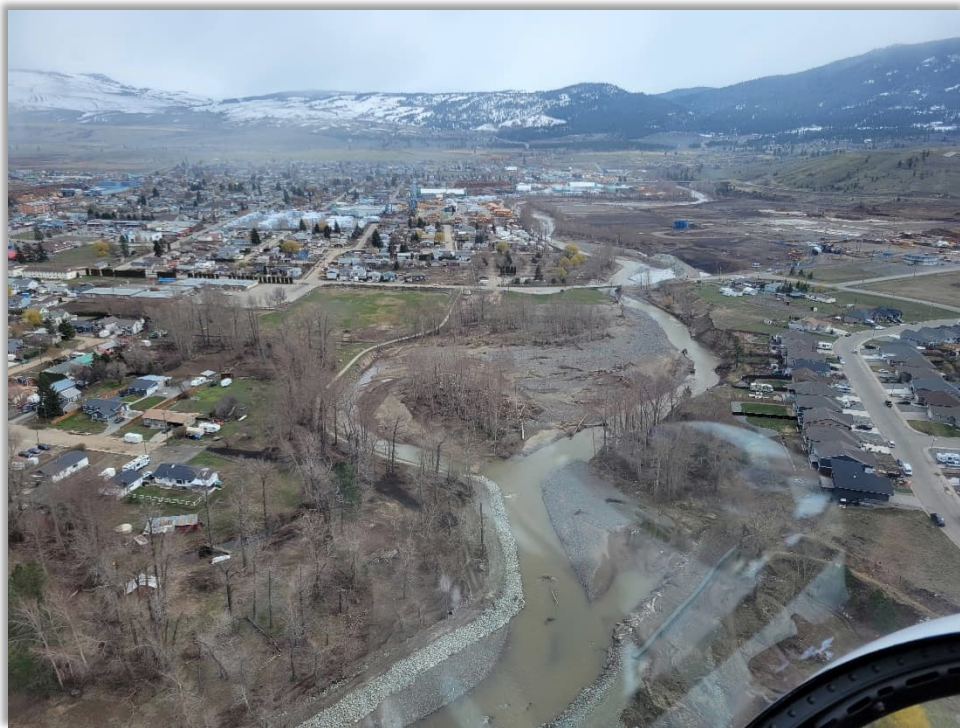
Aerial view of Coldwater River facing upstream near Chapman Street (left) and Fir Road (right), where channel avulsion occurred. The Middlesborough Bridge is visible upstream.
